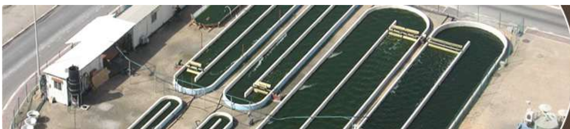
Figure 6 : Système de production ouvert de type Raceway. (Source : http://www.seamibiotic.com/research/microalgae-speices )
